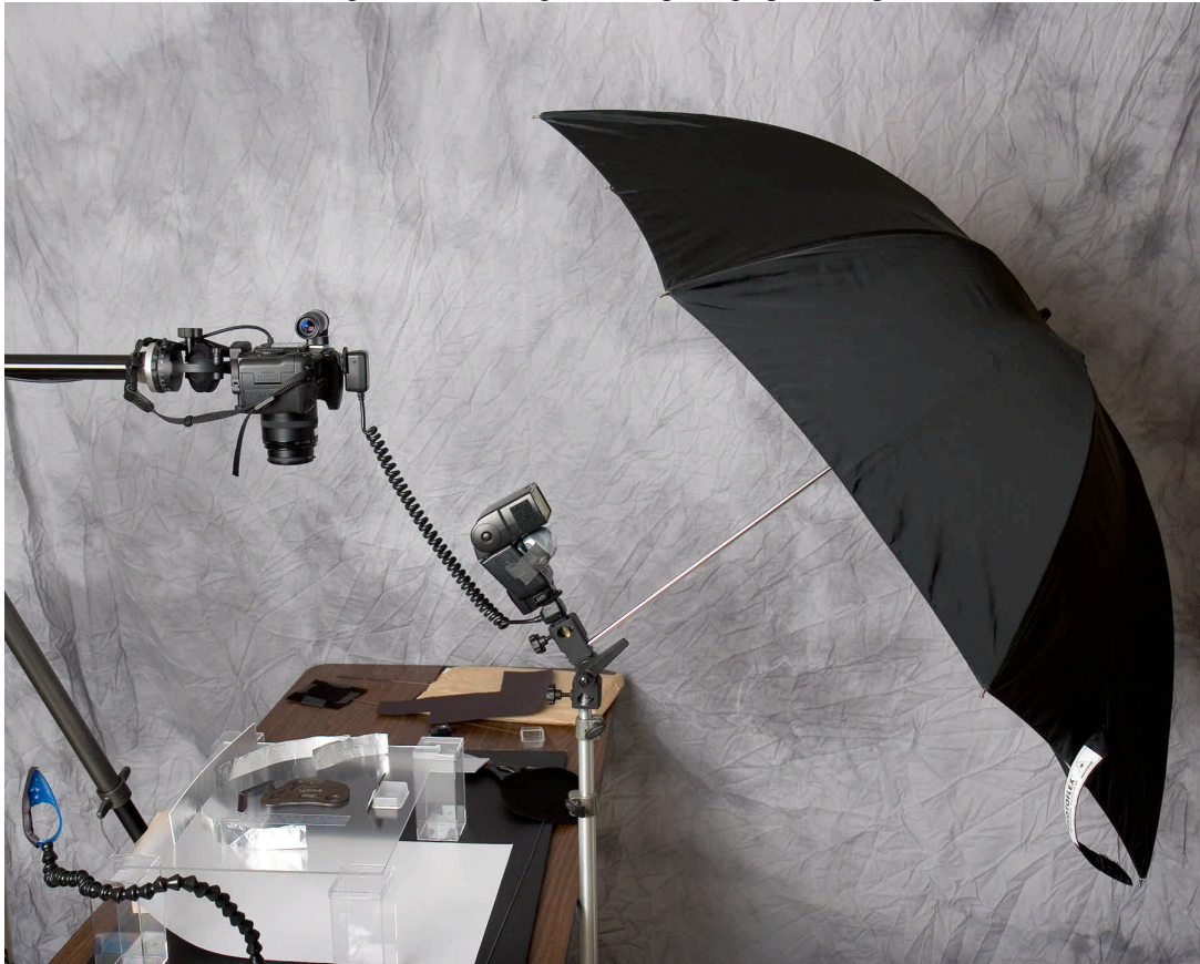
Figure – 4: “one light” flash photographic setup
